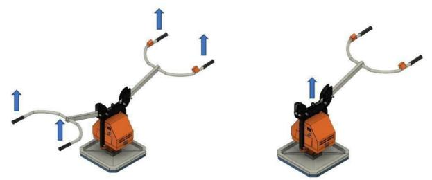
11. Position the handled element. To suck off – press both buttons on the machine handles at the same time.
