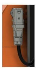
5. Connect the power cord plug to 110 V mains supply (do not use extension cables without earthing!). The mains or a power generator must be equipped with a residual current circuit breaker. Failure to follow these instructions may result in electric shock!!!
