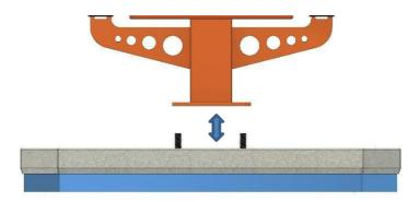
3. Before fitting the new suction cup, check the sealing between the suction cup and the machine and verify that the sealing profile under the suction cup is not damaged/worn.
