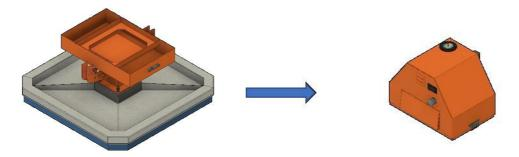
7. Clean the dirty filter with compressed air. You should also clean all vents with compressed air, as dust that is not removed will stick to the turbine, causing it to fail. Systematic cleaning will keep all electrical and mechanical elements in the best possible condition and reduce their failure rate.
