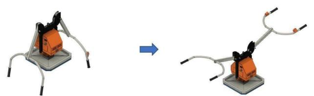
4. Connect the handle control connector to the machine (if not already connected).
